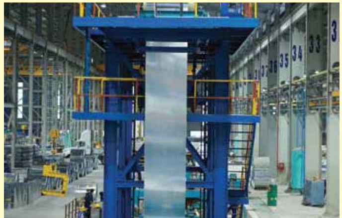
Galvanizing line (NOF technology – for galvanized steel sheet (GI)/ galvalume steel sheet (GL))
