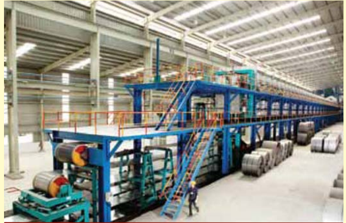
Hot galvanizing line (NOF technology – for galvanized steel sheet (GI)/ galvalume steel sheet (GL))
