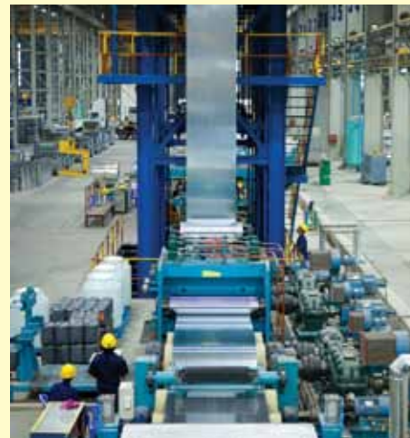
Galvanizing Steel line
